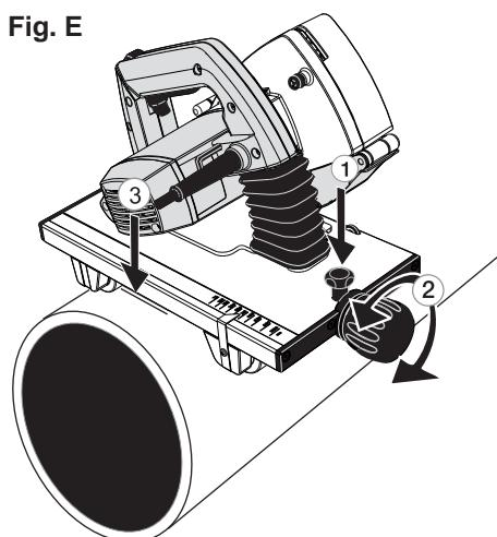
It is most important that the base of the steering device does not touch the pipe but rather that the wheel pairs support the saw (**Fig. E3**). Finally lock the adjustment with the safety screw (**Fig. E1**) so that the adjustments do not alter during the sawing.
