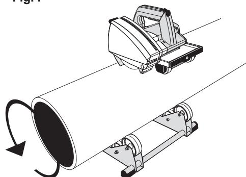
When the pipe is cut off, push the UNLOCK button forward until the yellow mark is visible and the locking is released (**Fig. L**). Now raise the motor unit to starting position. Release the power switch. After the saw is lifted away from the pipe ensure that the moving blade guard has turned into safety position (**Fig. M**).
