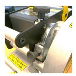
After the cut, pull cut / bevel locking pin to release the saw from down position. If settings are not modified, the saw will work the same on pipes with similar dimensions.
