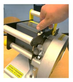
Begin the cut by pulling the yellow top locking pin to release the saw from up position. Pierce the pipe wall and push the saw down until the cut / bevel locking pin locks into the groove in counterback. Now you can fine tune the cutting depth / bevel width by turning the adjustment knob on top of the machine.
