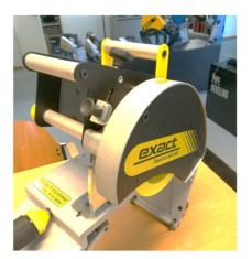
Depending on the pipe dimensions and bevel width, you may need to adjust the angle of the machine. Bevelling forces the machine to turn left from the operator point of view. To overcome this force, you may need to turn the machine a bit to the left on the gripper. Loosen the two screws, turn the bodyplate and tighten the screws.
