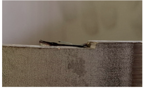
Incorrect cut (zoom in)
